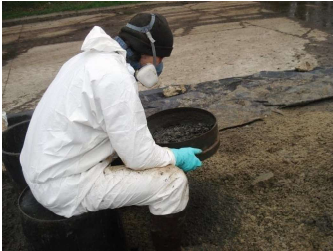
Manual sand sieving (Source: Le Floch Depollution)
