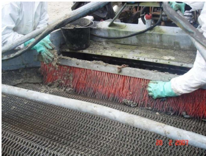
Mechanical sand/gravel/pebble sieving (Source: Le Floch Depollution)
