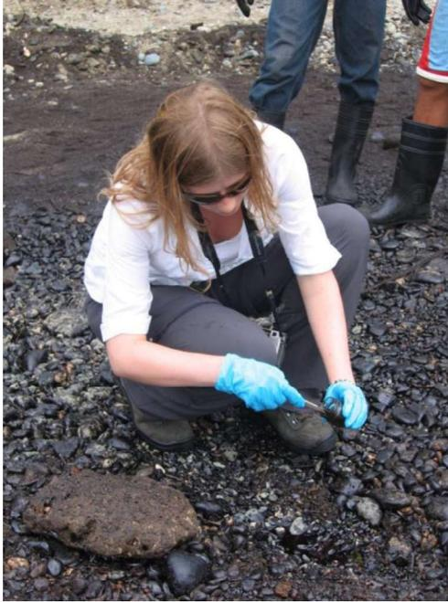
Sampling of OSW in glass container for analysis (Source: ITOFF)
