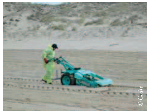
Mechanical selective sand screening
