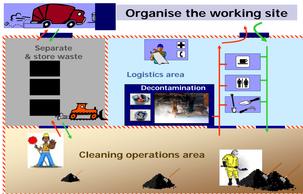
Figure 8 : Organisation of shoreline clean-up working site
