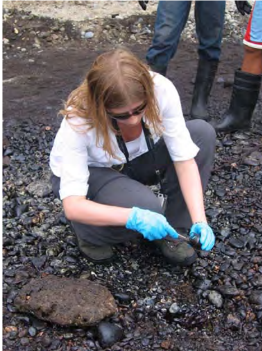
Sampling of OSW in glass container for analysis (Source: ITOPF)
